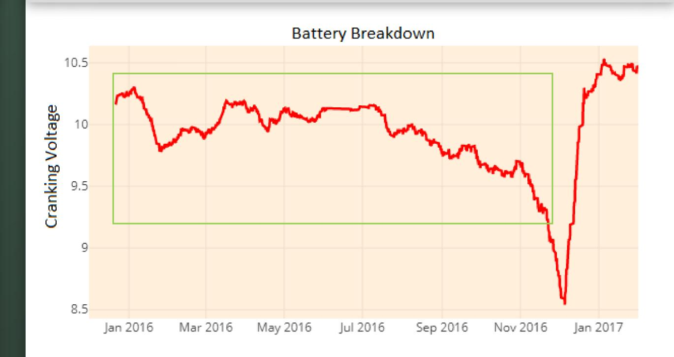
We have developed a Machine Learning model that can learn from historical battery breakdown curves and generalize rules that define a failing curve pattern. The model is trained only on the data points up to few days before the failure so that it can detect similar patterns to predict battery failures.
