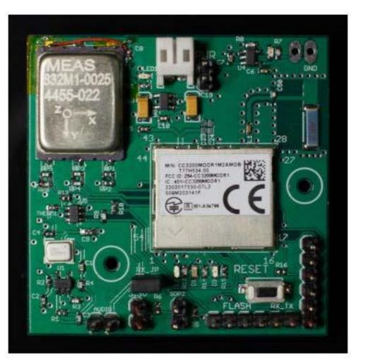
A sensory system is to be used to enhance the fault detection capabilities using sensors such as accelerometer and microphones. Accelerometer will capture the vibration and the microphone will capture the noise that may or may not be noticed by the driver. With the sensory system installed on the engine, numerous tests will be performed to obtain noise and vibration signals that represent healthy or faulty engine.
