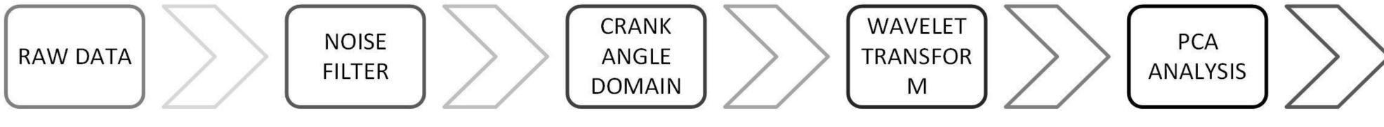
Collection of the raw data Filtering background noise from all analog sensory to improve the accuracy of the final results
