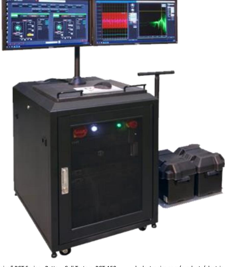
"D&V Electronics." BCT Series - Battery Cell Testers: BCT-150, www.dvelectronics.com/products/electricpowertrain-battery-testers/product-capabilities/specialty/bct-150-battery-cell-tester.html.
