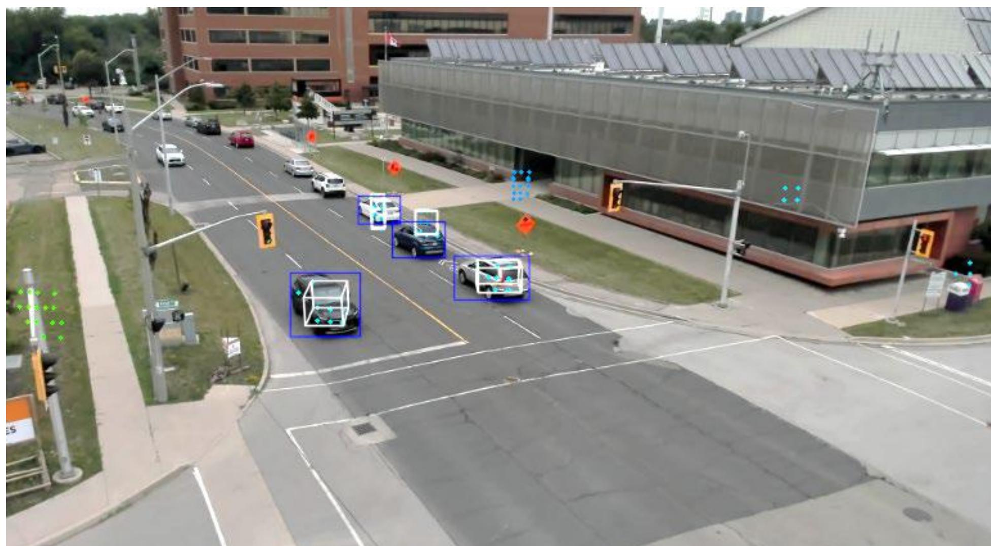
Objects are detected in the radar point cloud output and projected on the camera plane
