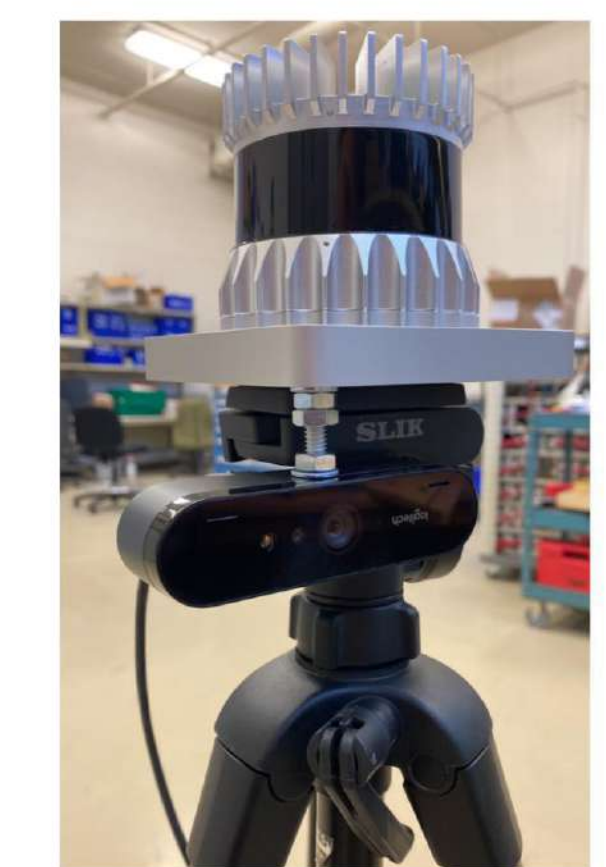
Figure 7. The Ouster OS1-64 used for data collection with a synchronized camera for future work.
