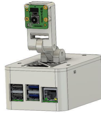
Figure 2. Raspberry Pi and camera mounting model.
