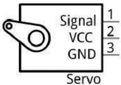
Figure 7: Pin description of Servo Motor
