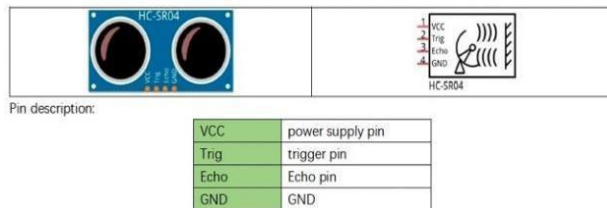
Figure 3: Pin description of Ultrasonic Ranging Module
